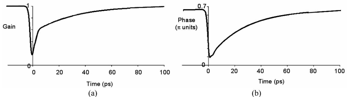
Figure 1. Typical (a) gain and (b) phase response of an SOA to a  $\sim 2$  ps optical pulse
