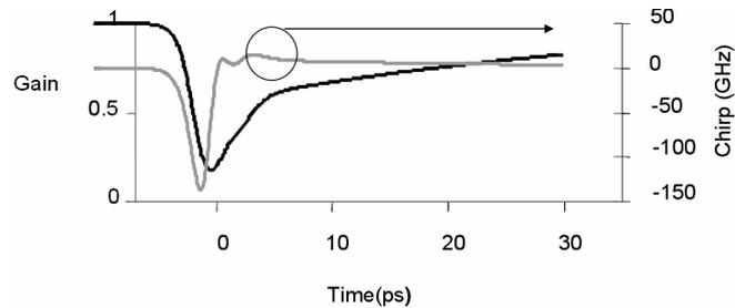
Figure 2. Gain (black line) and frequency shift (grey line) corresponding to the phase shift of Fig. 1.
