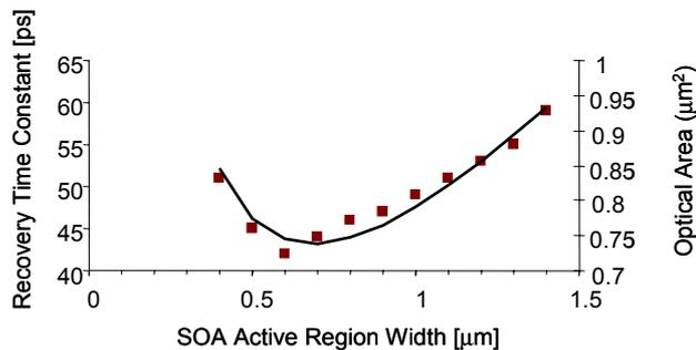
Figure 7. Modelled recovery time constant as a function of active region width (points), and modelled area to confinement factor ratio (solid line) overlaid for comparison.
