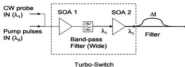
Figure 4. Turbo-Switch scheme. A DISC filter is placed after the Turbo-Switch for wavelength conversion.
