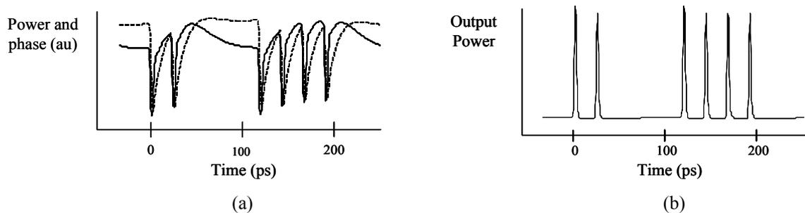
Figure 6. (a) Power output (solid line) and phase (dashed line) from the Turbo switch. The reduction in phase change for successive pulses is compensated by larger optical power (b) Power output from interferometer.
