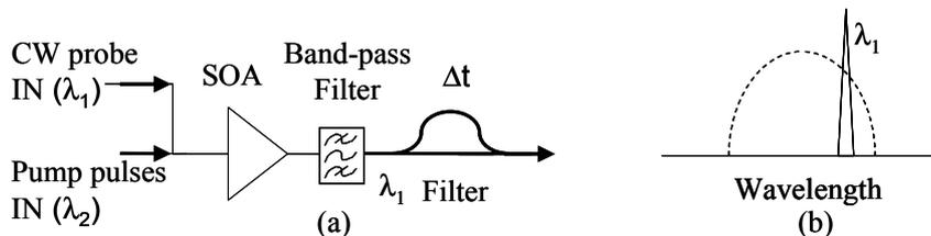
Figure 3. (a) Use of a pass-band filter and DISC filter to pass parts of the modulated CW probe spectrum [1]. (b) Placing of the CW wavelength to the blue side of the filter pass-band (dotted line).
