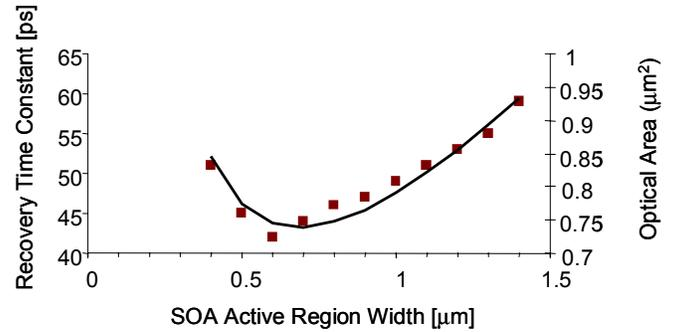
**Fig4.** Modelled recovery time constant as a function of active region width (points) and modelled area to confinement factor ratio (solid line) overlaid for comparison.
