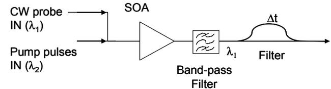
**Fig 1.** Use of a pass-band filter and ‘DISC’ filter to pass parts of the modulated CW probe spectrum (after Liu et al [1])
