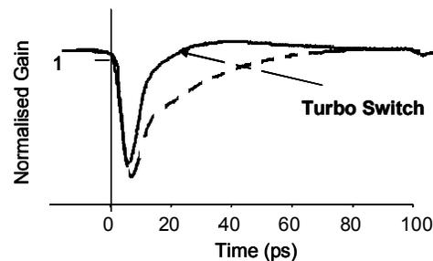
**Fig 3.** Measured response of the Turbo-Switch to a ~3ps pulse (from [6]). The slower response (dashed line) is for a single SOA.
