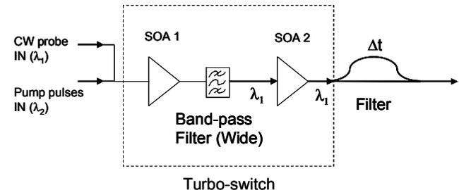
**Fig 2.** Turbo-Switch scheme. The band pass filter blocks the pump and allows the entire modulated CW spectrum to pass.
