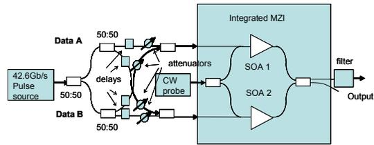
Fig. 1 Experimental setup for the hybrid integrated MZI XOR gate.
