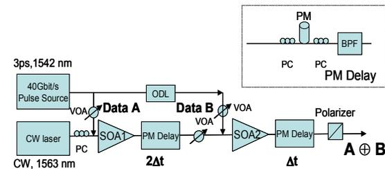
Fig. 2 Experimental setup of the DUX gate. Details of the PM delays shown in insert. PC: polarisation controller, PM: PM fibre, BPF: band-pass filter, VOA: variable optical attenuator, ODL: optical delay-line.
