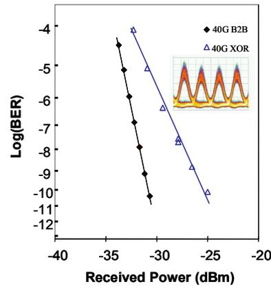
Fig. 4 BER for the DUX gate at 42.6Gbit/s with corresponding eye diagram (insert).
