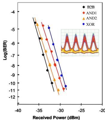
Fig. 3 Hybrid integrated XOR gate BER at 42.6Gbit/s with corresponding eye diagram (insert). Also shown, BERs for A and B separately (AND1 and AND2) and back-to-back measurement (B2B).
