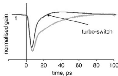
Fig. 3 Normalised gain measurement of CW beam modulated by one single 3ps control pulse shot
