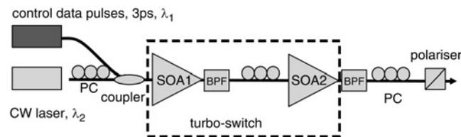
Fig. 2 Experimental setup of 40 Gbit/s wavelength converter using polarisation rotation
