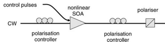
Fig. 1 Schematic of all-optical switch using nonlinear polarisation rotation in SOA
