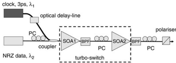
**Fig. 4** Experimental setup of NRZ to RZ format conversion
